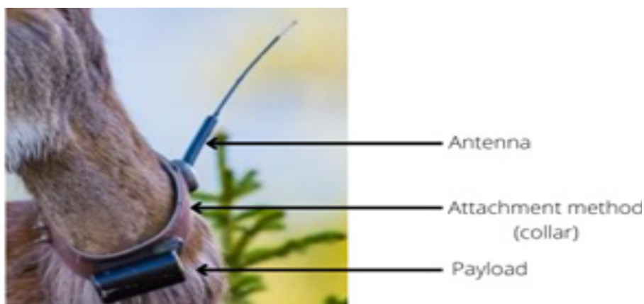
Figure 2. The three main components of a satellite tag. In this instance a GPS collar on a deer species.
